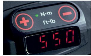
Torque setting adjustable per 10 Nm
