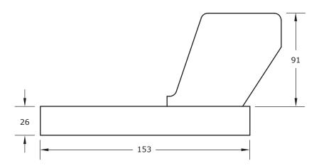
**ARTICLE:** ARTICLE NO: **SUITABLE FOR: RA 2400 NOSE X1=75 X2=165 Y=91 SPLINE**
